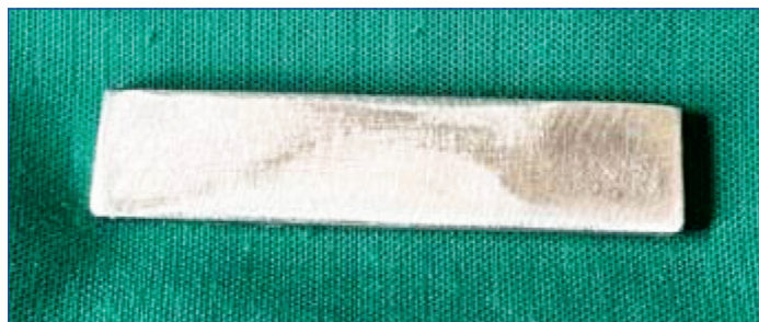
[Table/Fig-2]: Stainless steel die.
